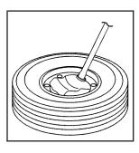
Tilt the retainer when the tire has been lowered, and slide it up the cable so it can be pulled up through the wheel opening.
